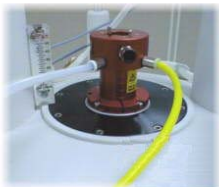
Figure 3.3. Magnet with BOSS Shim System Already Mounted
